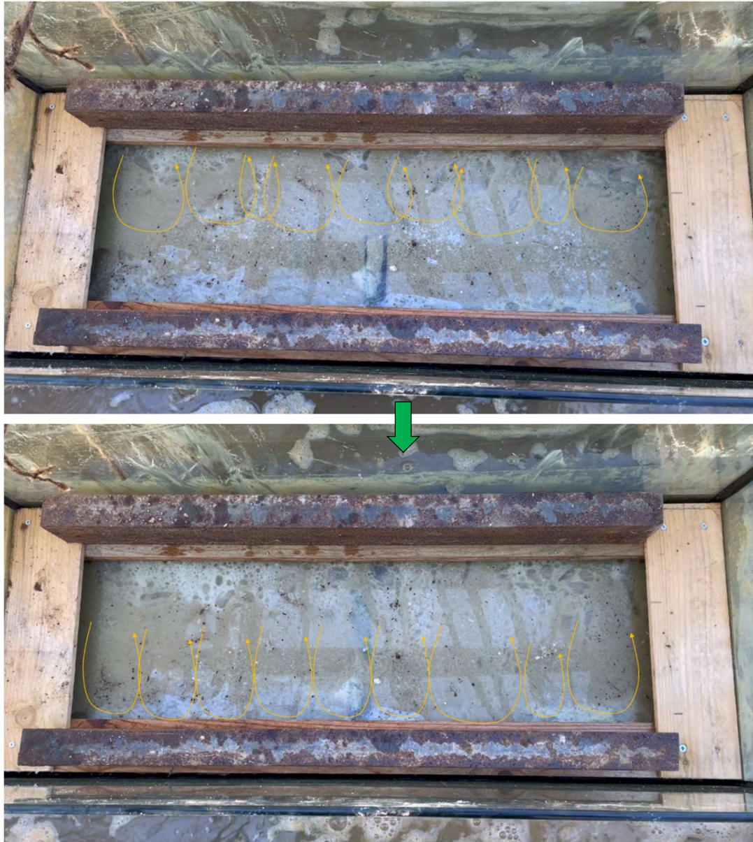
Figure 89 : Phase 1: jets going to their maximum range
