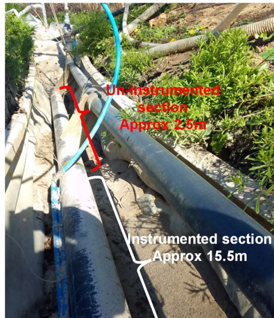
Figure 98: sketch of instrumentation along the pipe
