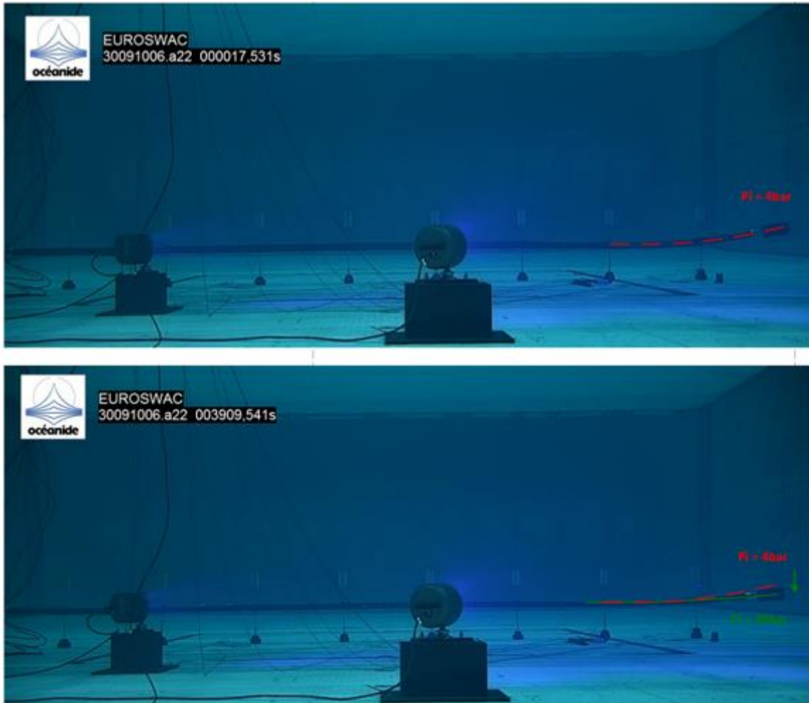
Figure 3-11: Experimental setup of test 14 – Bending stiffness test on Configuration 1 at P_i = 4\text{bar} and P_i = 40\text{bar} .
