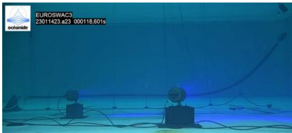
Picture 4-8: Flexible pipe system static state with AS 8 removed (test excluded of the test matrix).
