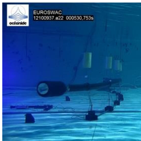
Picture 3-11: Transversal view of the flexible pipe system Configuration3 with the visible bend shape of the flexible pipe system under the action of a 90° heading REG2 (test 76).
