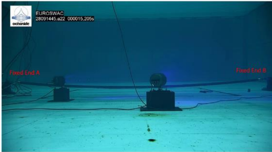
Picture 3-4: Test 1 – Axial tension characterization for P_i = 4.24\text{bar} and tension = 310.7kN.
