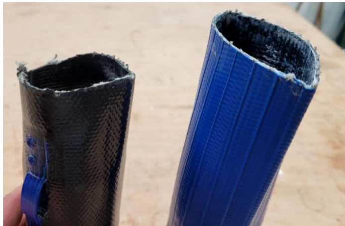
Picture 4-1: Pipe A retracting under pressure (left-hand side) and pipe B elongating under pressure (right-hand side).
